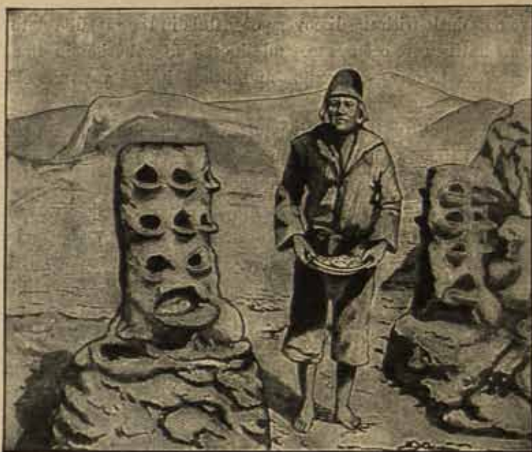
FIG 4.—LEAD SMELTING FURNACE, CENTRAL BOLIVIA. (From Archæologia , LVII, p. 363, by kind permission of the Society of Antiquaries.)
