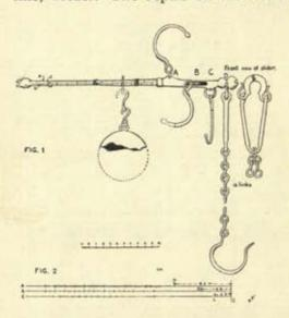
that it has made the arm nearly a quarter of an inch longer than it should be. The scales are cut on three edges of the arm, which is of diamond section. Scale A is divided into halves and twelfths; scale B into halves; scale C has equal divisions throughout, Fig. 2 shows the three scales, side by side, the error due to the length of the arm having been eliminated.
