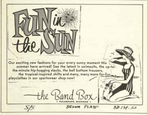
Fig. 38. Mechanical for two-color job. This is brown plate; S/S symbol indicates it is to be reproduced same size. Shadows have been exaggerated to distinguish various elements. Before plate-making they must be opaqued out.
