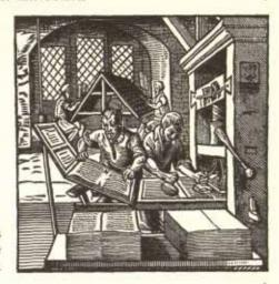
Fig. 3. Ancient printing press. Form is being inked by balls as printed sheet is removed. Typesetters in background.
