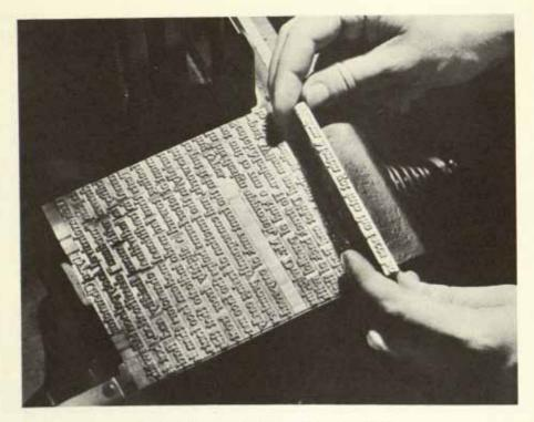
Fig. 27. Linotype slugs in galley on machine.
