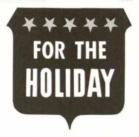
To create it, the engraver needs a negative on which type is black on a clear background. This he obtains by exposing the original negative —with clear type on black—onto a second piece of film. From this reverse negative the plate is made as any other line cut.
