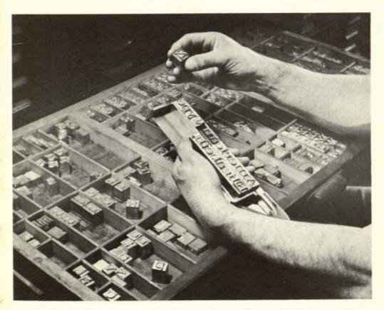
Fig. 24. Setting type into composing stick from California job case. (Courtesy American Type Founders)
