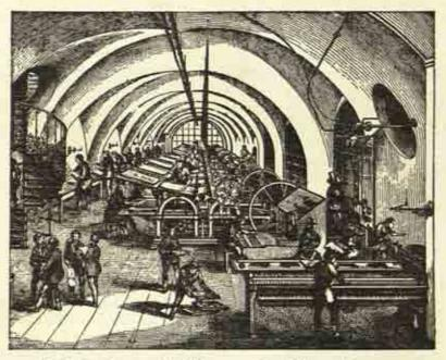
48. In the foreground of this engraving of the machine room of the State printing house in Vienna about 1840 are a typedistributing machine and a type-setting machine with a piano keyboard of 120 keys.
