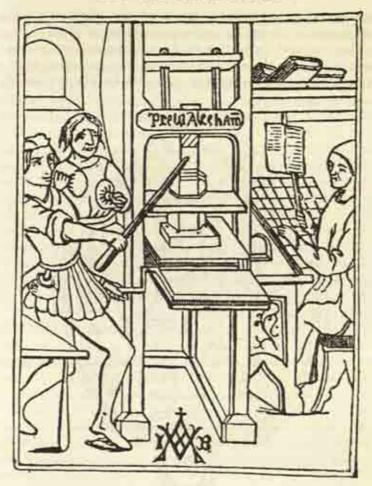
28. An early printing press, from a wood-cut dated 1507. In the background is a compositor with his copy on a stick and his type case before him. The pressman's assistant manipulates a pair of ink balls. The press is braced to the ceiling, but it is light in construction. Other illustrations show presses of much heavier build.
