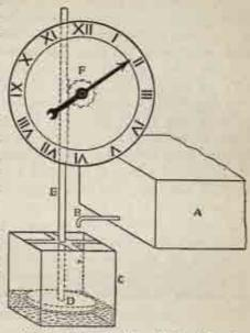
Fm. 31. Water clock described by Vitruvius. From the tank A water drips at a uniform rate through the small pipe B into the reservoir c in which is the float D. From the upper surface of D rises the shaft E the teeth of which, by their movement as the shaft rises, rotate the cog-wheel F. To this cog-wheel is attached a hand the position of which, on the surface of the dial, indicates the hour.
