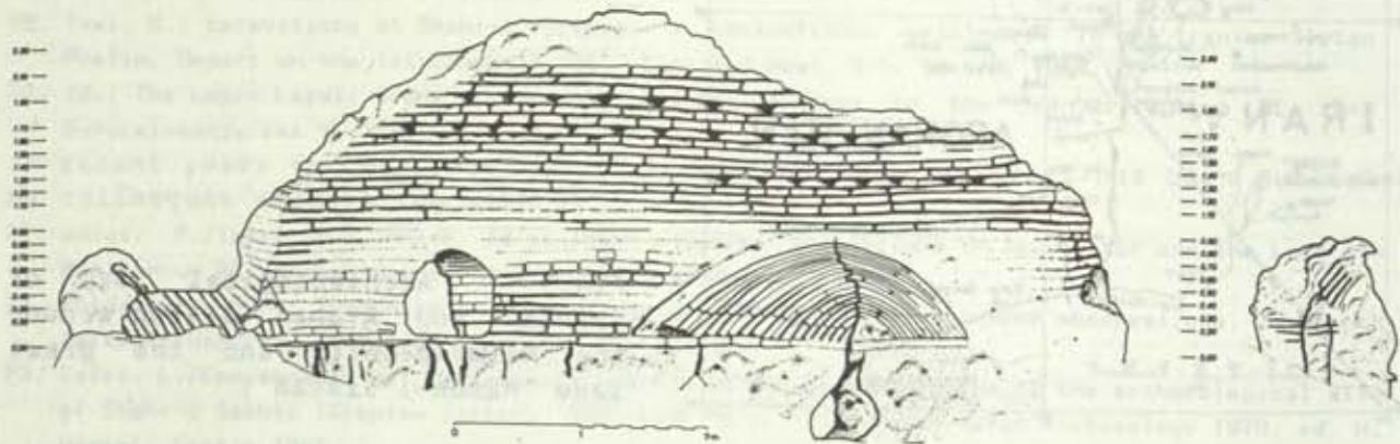
Fig. 4 Photogrammetric interpretation of building 8 on the plan of Dewal-i Khodaydad (see Fig. 2): transition from square ground plan to coupola by squinches. Drawn by the Institute of Photogrammetry, Bonn University
