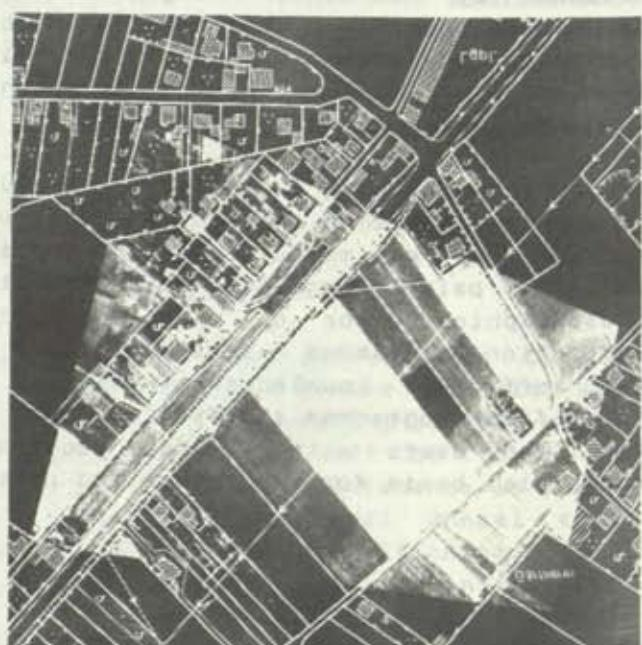
Pl.2B Orthophoto with superimposed 1:5,000 German Base Map of Centre of Pl.2A. Digital Interpolation with bicubic spline approximation to Sinc function following Simon.
