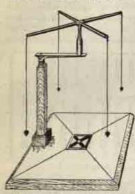
Fig. 18. The Groms: Reconstructed from descriptions, remains, and ancient representations.
