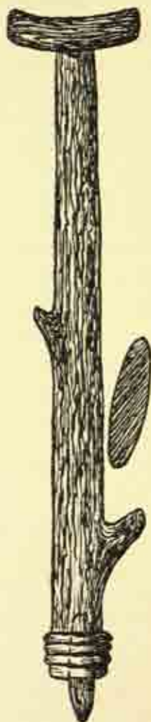
FIG. 24. Wooden flaking-staff pointed with walrus-tusk, for impulsive-pressure-plus-percussion. The branch on the left side was used to secure a heavy stone. The cross-piece is against the operator's chest, and when he throws his weight on it, an assistant gives a sharp blow in the crotch on the right-hand side with a wooden club of oval section shown on the right of the staff. Drawn by I. M. Allen from the sketch and description by G. E. Sellers, Ann. Rep. Board of Regents, Smithsonian Inst. , 1885, p. 875.
