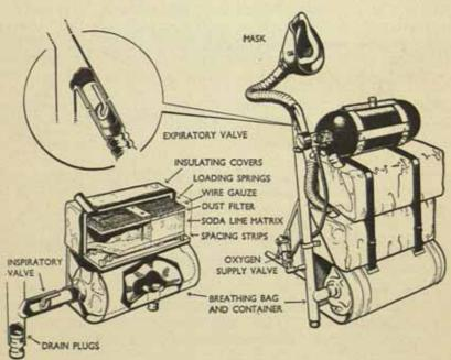
Fig. 3.—Closed-Circuit Apparatus.
